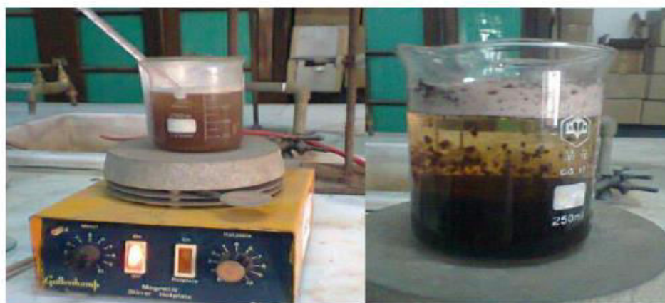
Fig 1: Hydrolysis of jute using 64% w/v H 2 SO 4 for preparation of cellulose nanocrystals (left: initial stage, right: after hydrolysis).
