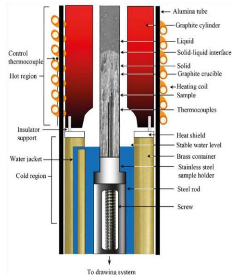
**Fig. 1:** Bridgman furnace scheme (Douglas, 2020).
