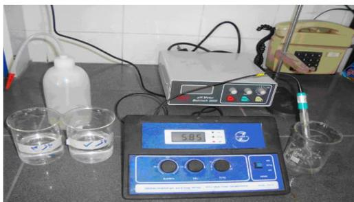
**Fig. 5:** Image of pH meter device.
