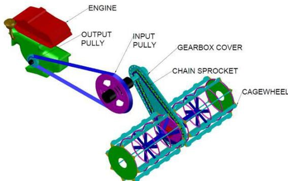
**Fig. 7:** Power transmission system of Hydro tiller.
