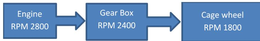
**Fig. 6:** Flow sheet diagram of power transmission system of the modified hydro-tiller.
