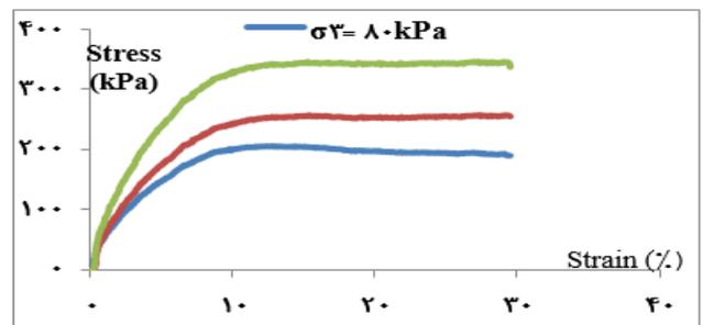
**Fig. 9:** Stress-strain curve of uniaxial test for 6% plastic bottle as.
