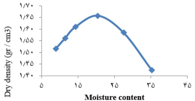
**Fig. 3:** Clay density curve.
