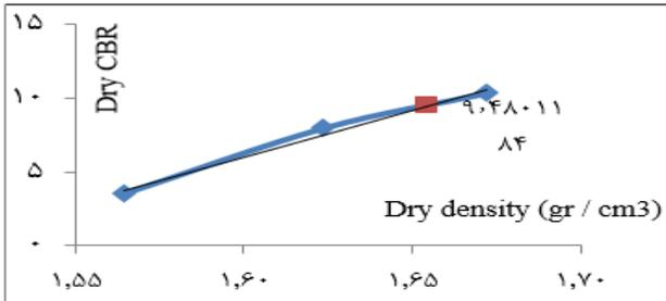
**Fig. 5:** CBR graph of soil dry density.
