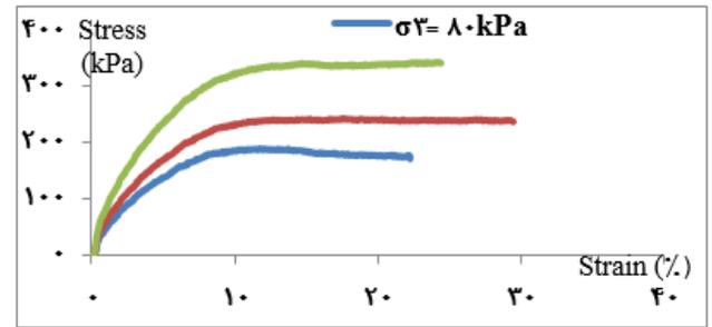
**Fig. 8:** Stress-strain curve of uniaxial test for 3% plastic bottle ash.
