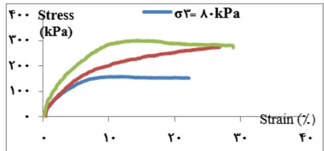
**Fig. 7:** Stress-strain curve of uniaxial test for 0% plastic bottle ash.
