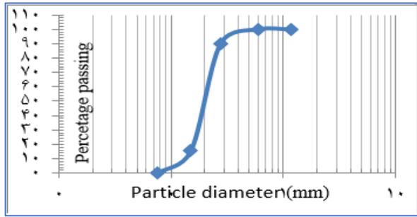
**Fig. 1:** Sandy soil gradation curve.
