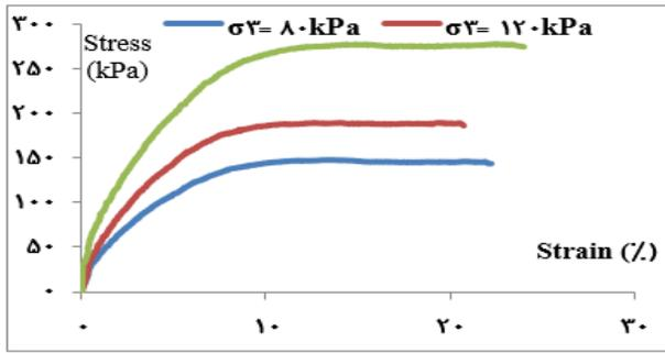
**Fig. 10:** Stress-strain curve of uniaxial test for 9% plastic bottle ash.
