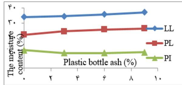
**Fig. 4:** Variation of Atterberg limits with different percentages of plastic bottle ash.
