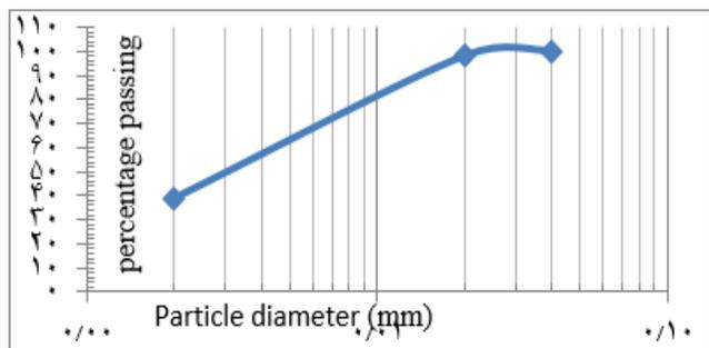
**Fig. 2:** Clay gradation curve.
