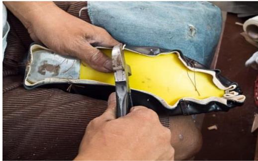
**Fig. 1:** Lasting process.
