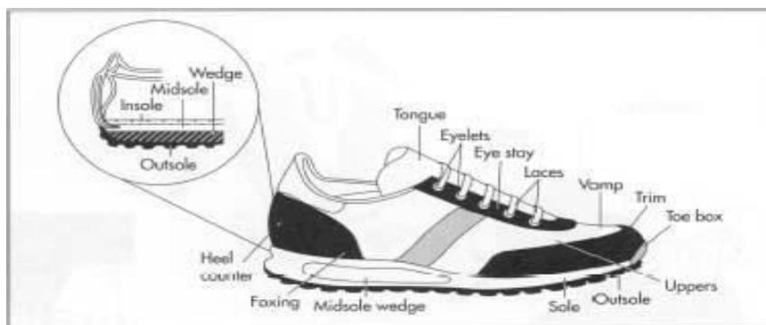
**Fig. 4:** Cemented lasted full shoe.
