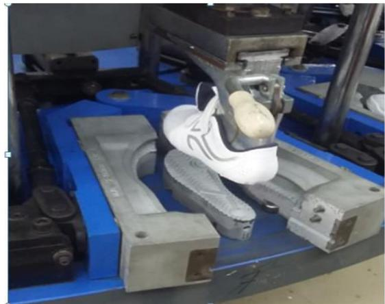
**Fig. 8:** TS 700 JR directly injected by TPR.
