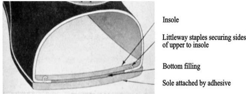
**Fig. 5:** Cemented lasting construction.
